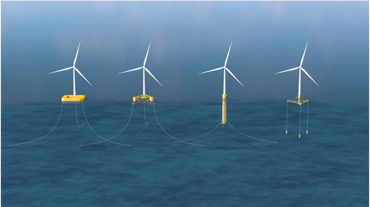
Figure 3.2: Potential Floating Foundation types considered for the Offshore Proposed Development (from the left, barge, semi-submersible, spar and tension-leg platform)
