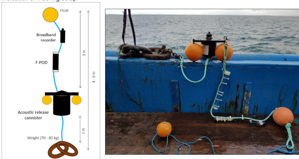
Figure 1 PAM mooring configuration
